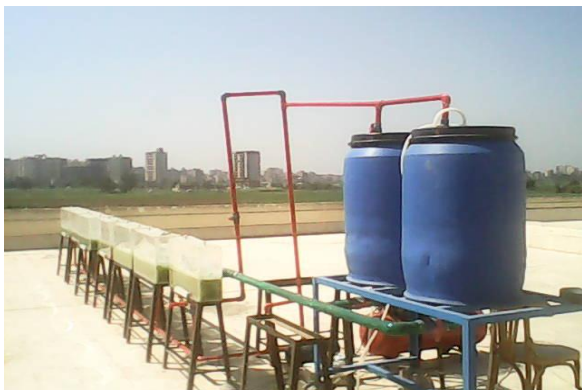
Fig.1. Cultivation system of S. obliquus at large scale showing the glass boxes. Each one contains 40L of moh202 media in the sun light with a photoperiod 14:10 h light: dark and aerated using air pump.
